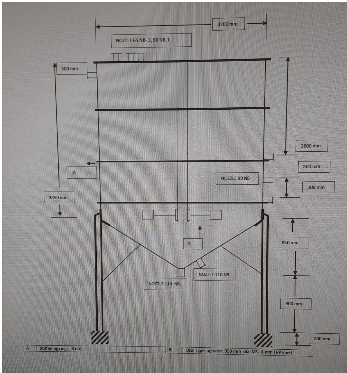
**30 M3 CAPACITY CONICAL BOTTOM MSFRP TANK (WITH GRIDS)**
