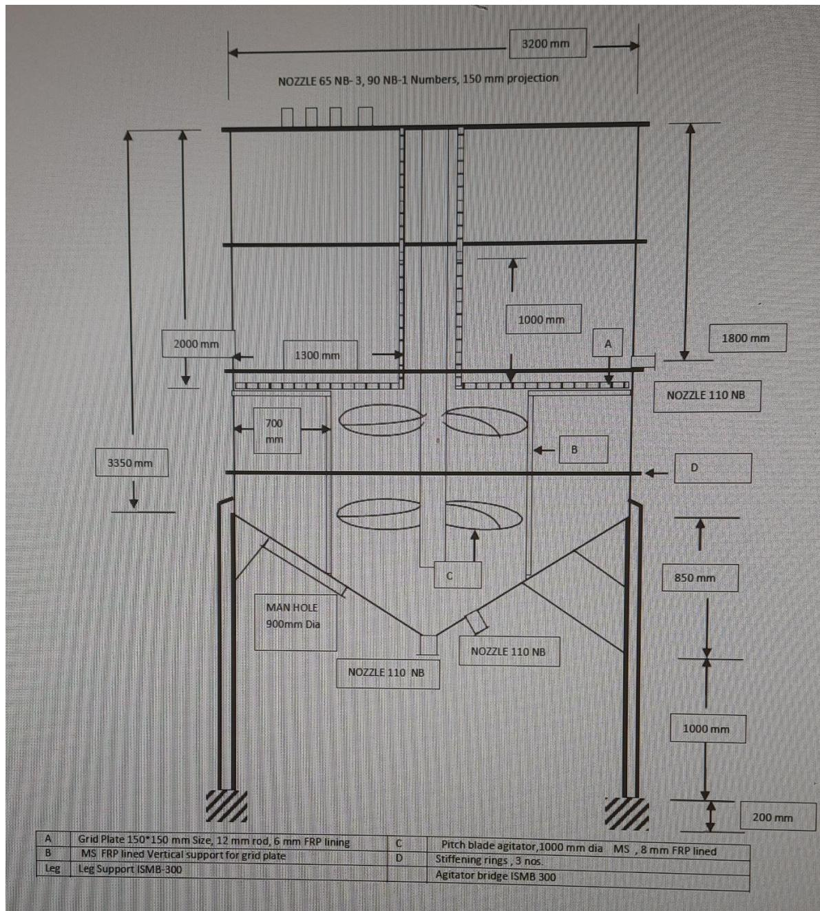
**1.5 M<sup>3</sup> CAPACITY CONICAL BOTTOM MSFRP TANK**
